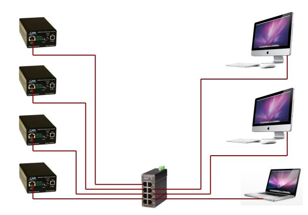
Figure 4.1: CANflight/Host Computer Communication Network
