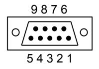
Figure 3.2: CAN1/CAN2 D-Sub Connector Pinout
