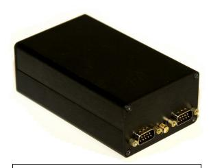
Uses Dual DB-9 Male Connectors for ease in wiring ARINC-825 / CAN busses. IRIG-B timing input also shown on SMA. SMA to BCN adapter available.
