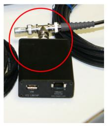
On the opposite end, plug one end of the USB cable into the port marked USB on the LANTAP, and the other end into your computer. *Please note, that ICS strongly recommends using a USB 3.0 port. These are usually blue instead of black or grey and provide up to 1 amp of current.*
