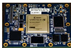
ASCB-D Airborne NIC and PROC in 6x10cm PWB weighing 70 Grams and using 2W.
